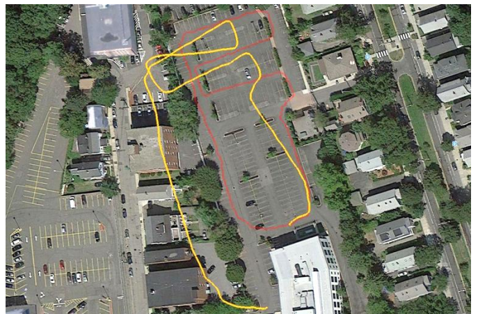
Fig. 5: Output of ekf_localization_node (orange) when fusing data from odometry and two IMUs. Note that the second IMU stopped reporting data midway through the run.
