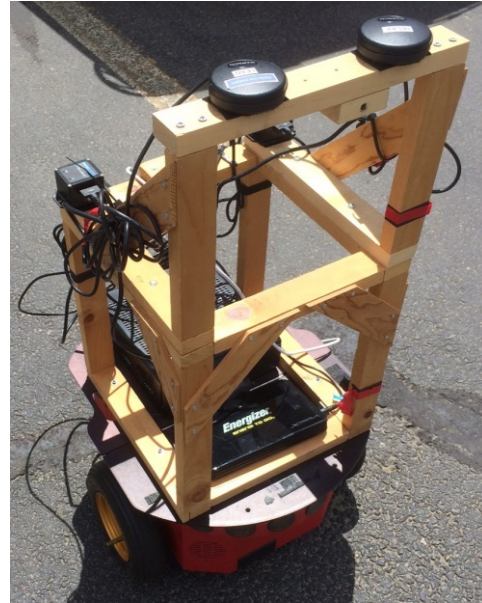
Fig. 1: Our test platform is a Pioneer 3 with a custom sensor mounting rack. It has two IMUs and two GPS units.
