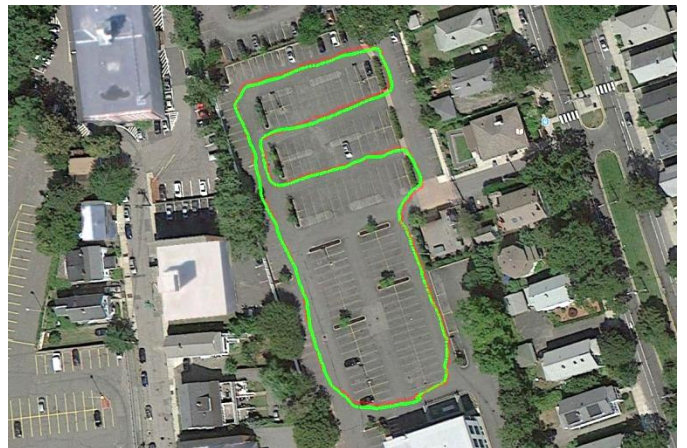
Fig. 7: Output of ekf_localization_node (green) when fusing data from odometry, two IMUs, and two GPS units.
